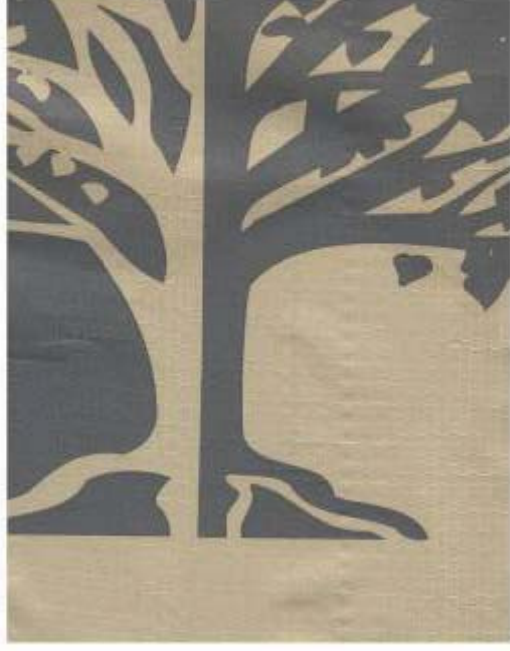
The Polypropylene (PP) woven(W) with matt lamination 100 Gr/M2
