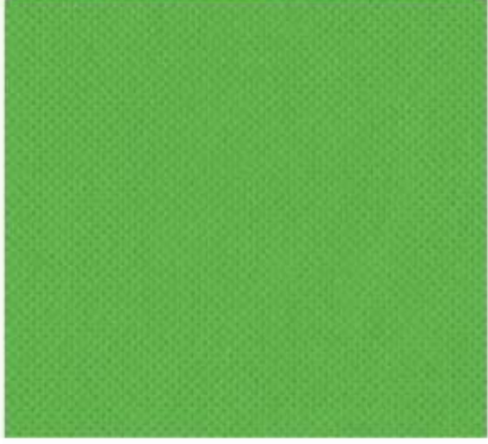
The Polypropylene (PP) non woven (NW) without lamination 80 Gr/M2
