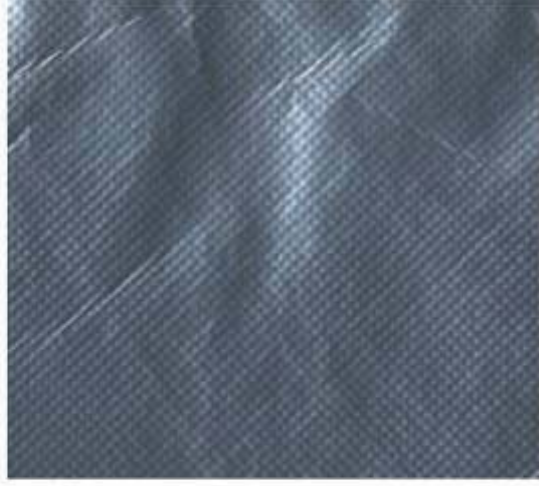
The Polypropylene (PP) non woven (NW) with matt metallic lamination 80 Gr/M2
