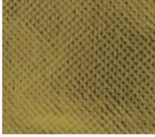
The Polypropylene (PP) non woven (NW) with shiny metallic lamination 80 Gr/M2
