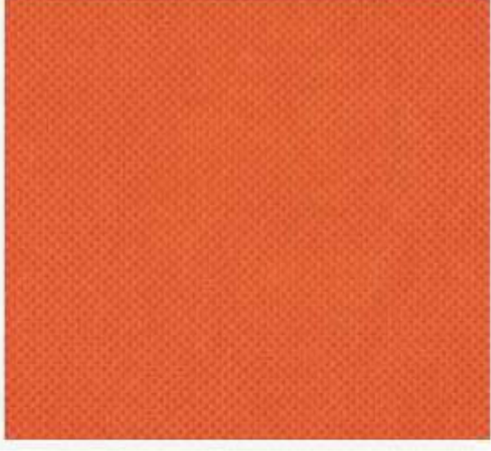
The Polypropylene (PP) non woven (NW) without lamination 120 Gr/M2
